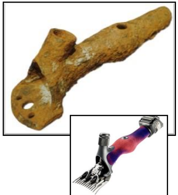
Old shearing handpiece found near sheep yards, and inset, modern handpiece for comparison
